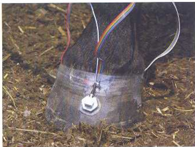
A close-up of the sensors attached to a horse's hoof in preparation for one of Dr. Jeff Thomason's studies of forces acting on the hoof wall.
